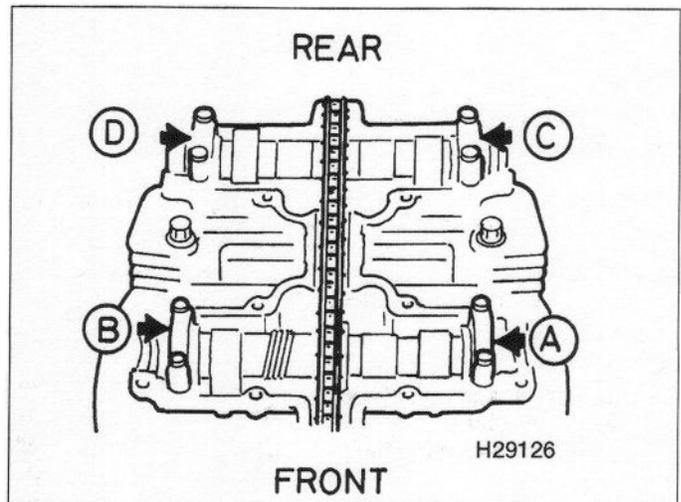
10.4 Camshaft cap identification markings
