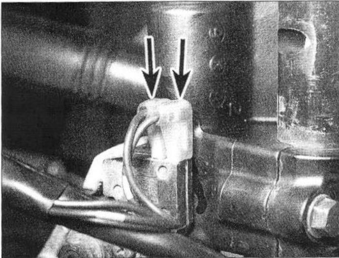
14.5 Front brake light switch wiring connectors (arrows)
