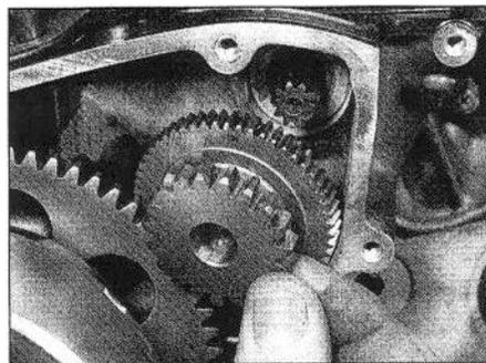
21.12a Install the idle/reduction gear . . .
