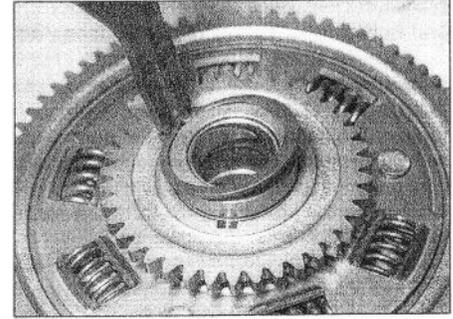
17.18c . . . and secure it with the circlip
