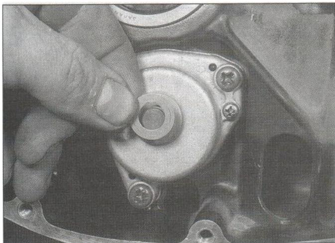
19.7a Slide the washer onto the shaft . . .
