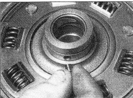
17.18a Fit the pin into its hole . . .
