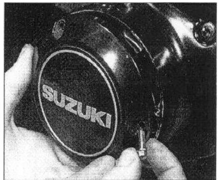
17.27 Install the pulse generator assembly cover
