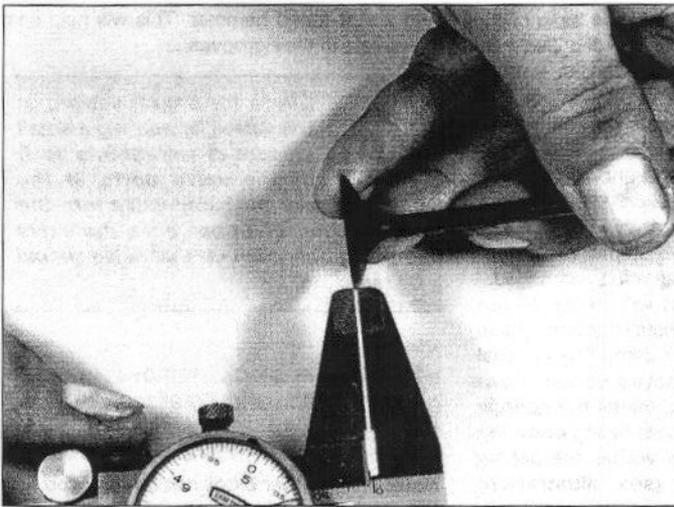
13.15 Measure the valve face thickness as shown
