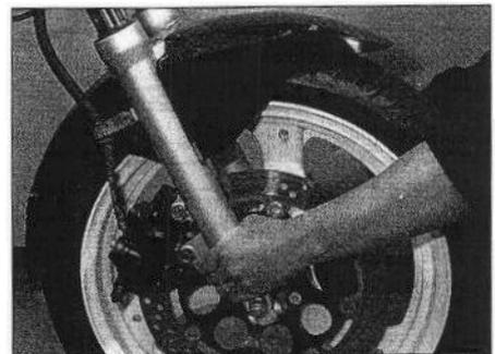
16.4 Checking for play in the steering head bearings
