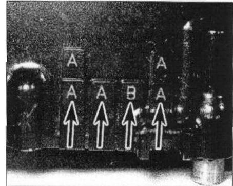
**29.10b Crankshaft main bearing housing size codes (arrows)**
