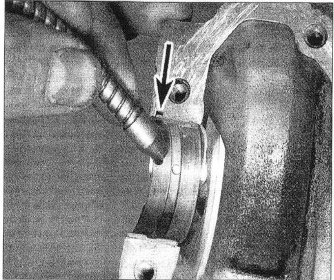
30.23b . . . making sure the tab locates in the notch (arrow), and lubricate them generously
