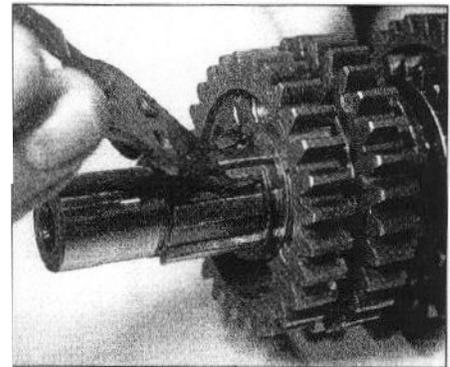
26.39c . . . and secure them with the circlip
