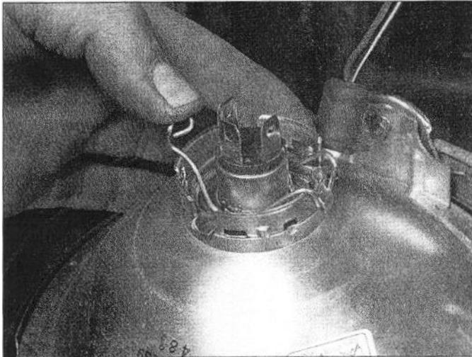
7.3a Release the bulb retaining clip . . .
