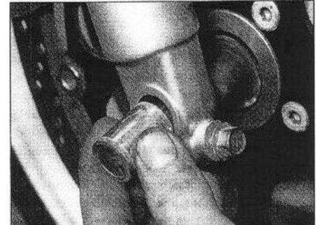
14.11b . . . and the axle spacer if removed
