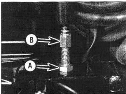
10.3 Locknut (A), adjuster (B) (clutch end)
