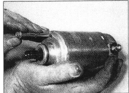
30.21 Install the long bolts using new O-rings
