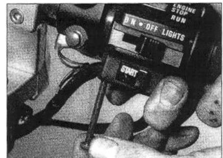
21.2 The switch is secured by two screws
