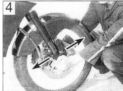
4 Checking the steering head bearings for freeplay
