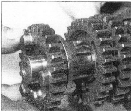
26.40a Install the 5th gear pinion . . .
