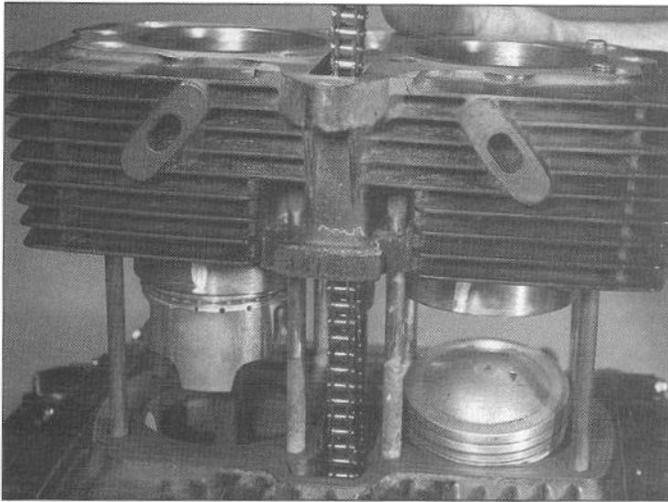
14.17 Carefully lower the block onto the pistons
