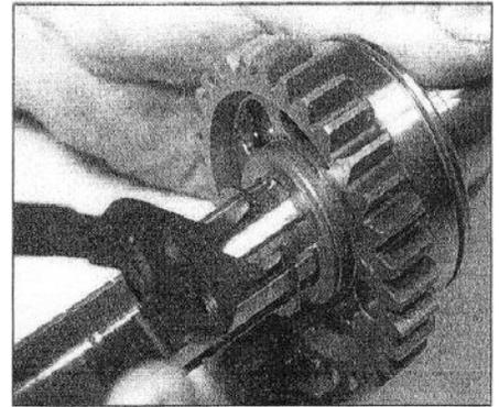
26.36c ... and secure them with the circlip
