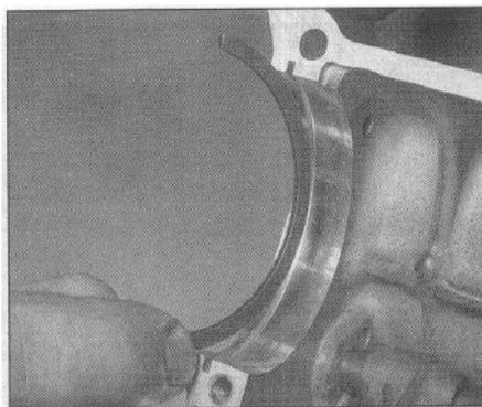
25.5a Fit the input shaft bearing retainer ...
