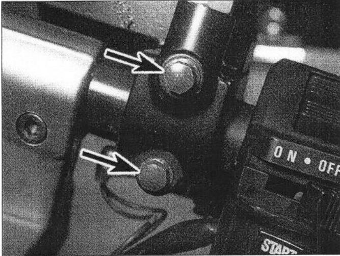
5.8 Front brake master cylinder clamp bolts (arrows)
