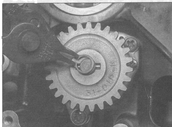
19.7d . . . and secure it with the circlip
