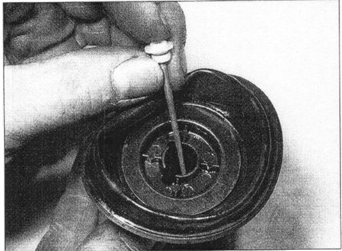
**7.5** Withdraw the jet needle assembly
