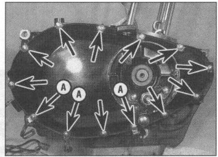
17.3 The crankcase cover is secured by thirteen bolts (arrows). Note the positions of the wiring clips on three of the bolts (A)
