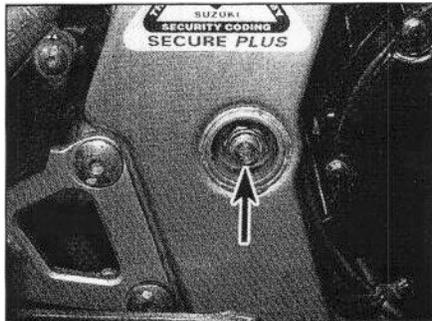
**13.6a Unscrew the swingarm pivot nut (arrow) ...**
