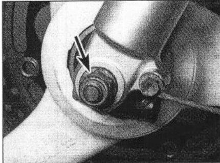
14.4b . . . then unscrew the axle nut (arrow)
