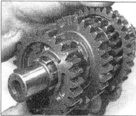
26.39a Install the 4th gear pinion . . .
