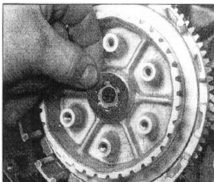
17.20c Slide lockwasher onto the shaft . . .
