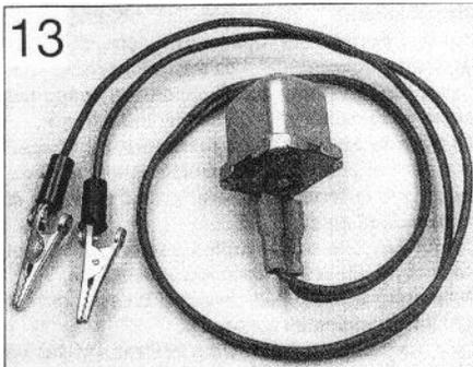
13 A buzzer is useful for voltage checks
