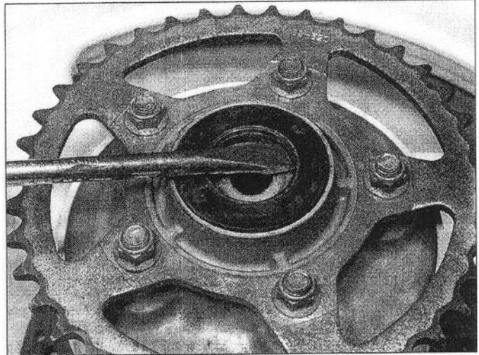
16.24b . . . then lever out the bearing seal
