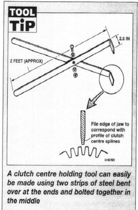
A clutch centre holding tool can easily be made using two strips of steel bent over at the ends and bolted together in the middle
