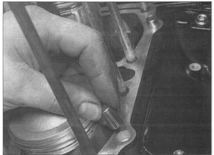
14.14 Install the dowels in the crankcase surface
