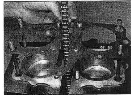
11.13a Fit the new cylinder head gasket . . .
