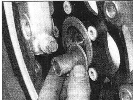
14.11a Install the wheel spacer as shown . . .
