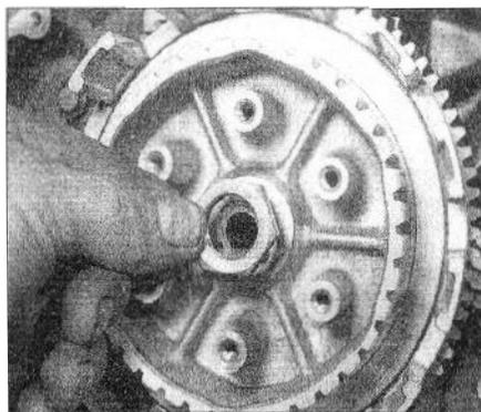
17.20d . . . then install the clutch nut . . .
