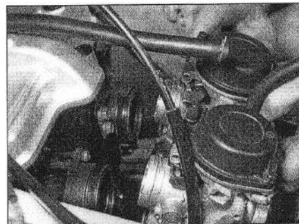
6.7b . . . and remove the carburettors
