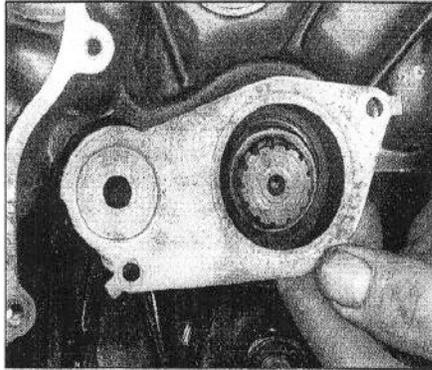
**23.22a** Install the output shaft retainer plate . . .
