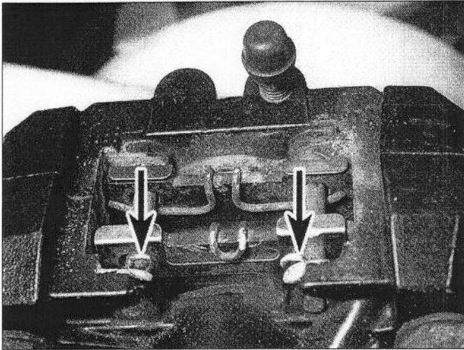
6.2 Remove the pad pin clips . . .
