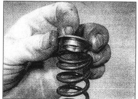
7.26b ... followed by the spring seat (make sure its shouldered side fits into the top of the spring) ...
