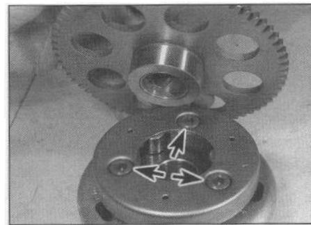
21.4b The starter clutch is secured to the back of the rotor by three bolts (arrows)
