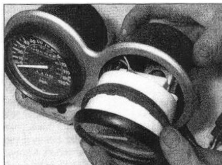
16.4a Withdraw the instrument from the casing ...
